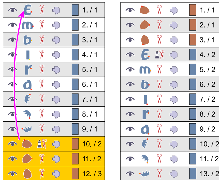
Fig. 20. Use drag-and-drop operation with primary mouse button to change sewing order of objects. Chose Insert Before option from the pop-up menu that appears. Picture at the right side shows the new order of objects.
