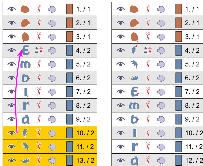
Fig. 21. Use drag-and-drop operation with primary mouse button to change sewing order of objects. Chose Insert Before option from the pop-up menu that appears. Picture at the right side shows the new order of objects.
